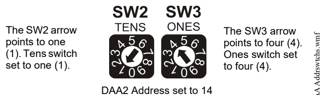
Figure 2.39 DAA2 Address Switches
